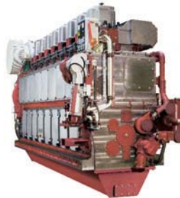
● M 32 C 6, 8, 9 cylinder 2,880–4,500 kW
