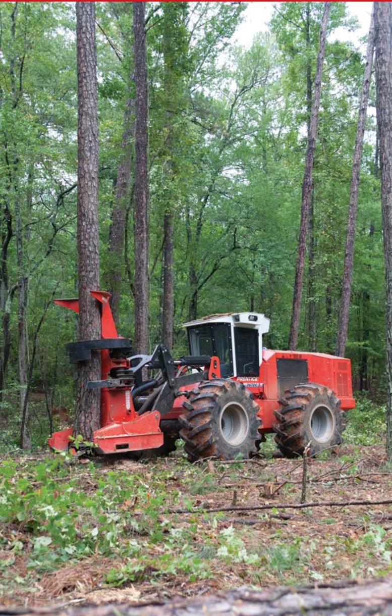
Unique operating modes, combined with complete electrohydraulic controls, provide the operator with a smoother machine with increased productivity. These modes include Terrain Selection Mode to optimize performance on hills or flat ground, Creep Mode to improve machine functionality, particularly in first thinnings, and Road Steer Mode for high-speed transport of the machine.
