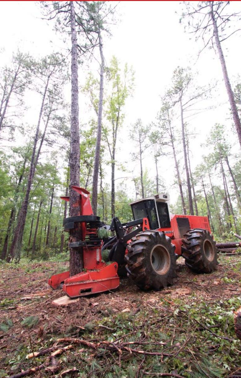
Cat engines, field-proven hydrostatic drive and Cat axles make a solid, responsive power train. A new design to keep the pump drive and gearbox well lubricated provides even more durability.
