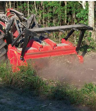
New work tools have been developed to match the powerful capability of the 2864C Site Prep Tractor. The Prentice MD-250 Mulcher and the Prentice MR-244 Brushcutter are available from the factory and supported by your Prentice dealer. Other key 2864C attachments include an attachment quick coupler and retrieval assist winch to increase versatility.
