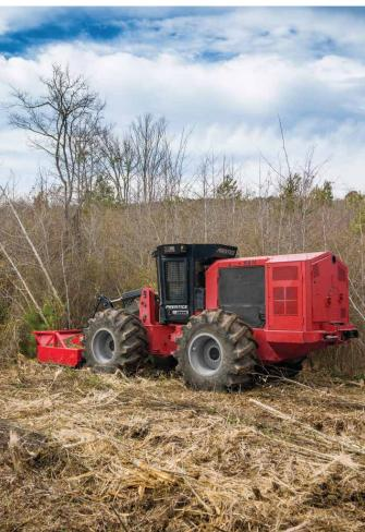
Unique operating modes, combined with complete electrohydraulic controls, provide the operator with a smoother machine with increased productivity. These modes include Creep Mode to easily adjust machine speed to improve mulching, Terrain Selection Mode to optimize performance on hills or flat ground, and Road Steer Mode for high-speed transport of the machine.
