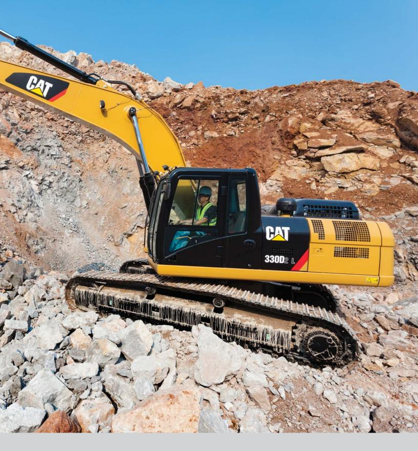
The 330D2 L comes with a number of new developments and features to help you make the best use of your machine including, isochronous engine speed control, a new fuel filtration system, a built-in economy mode to reduce fuel consumption. A variable speed fan with viscous clutch makes this machine productive, efficient, and safe.
