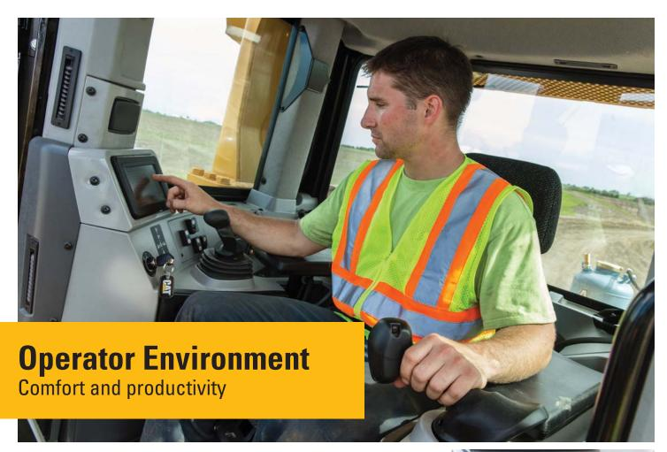
The latest D8T offers operators added comforts like a quieter cab, adjustable armrests and a heated/ventilated seat option. A seat belt indicator light helps remind you to work more safely.
