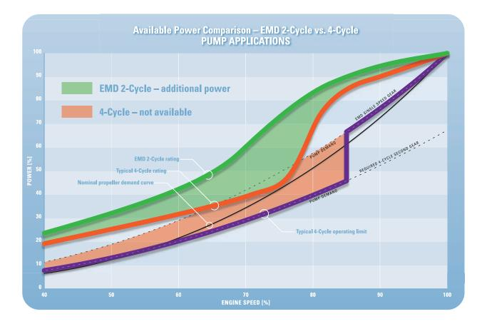
With abundant available power above the pump demand curve, the EMD 2-cycle engine is more responsive and productive with a lower cost single gear driveline. Typically, single gear driveline causes pump demand curves to exceed a 4-cycle engine's power rating at engine speeds lower than 85% of rated.
