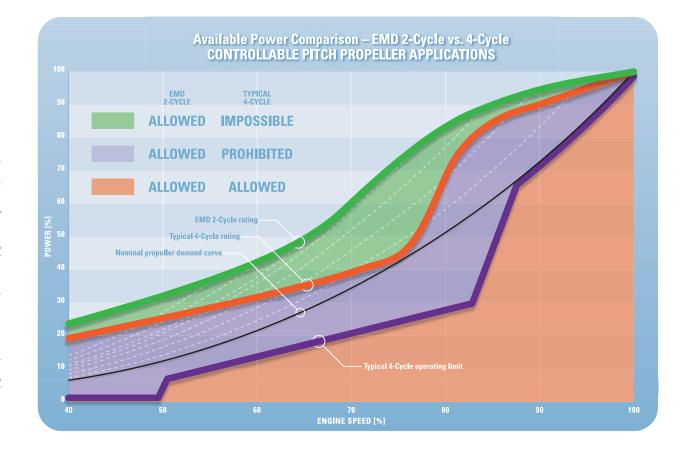
The additional power capacity of the EMD 2-cycle engine provides better responsiveness and allows operation at any point up to the continuous rating, enabling it to accept virtually any pitch at any rate without overload.
