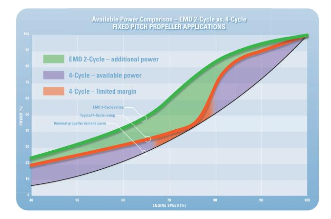
The EMD 2-cycle engine provides a large margin of available power above the demand curve to provide superior acceleration and responsiveness. By comparison, in fixed pitch propeller applications, the available power of a typical 4-cycle engine narrowly meets the propeller demand curve, especially in the middle to upper engine speed range. Load variations, due to changes in operating conditions, risk increasing the power demand into regions that can overload 4-cycle engines.
