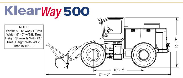
**Description:** The Klearway 500 is a rough terrain, rubber-tired vehicle with a front mounted rotary or shredder-type cutterhead designed to clear vegetation from utility right-of-ways, railroad right-of-ways and for site preparation.
