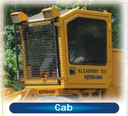
Angled front roof panel equipped with viewing window to allow easier positioning in utility right-ofway. Pilot-pressure joystick control for cutterhead tilt and lift functions. Tilt steering wheel with flow amplification steering. Selfcontained air conditioner/heater. Fully adjustable seat with suspension and belts. Large roomy cab with easy access and excellent visibility.
