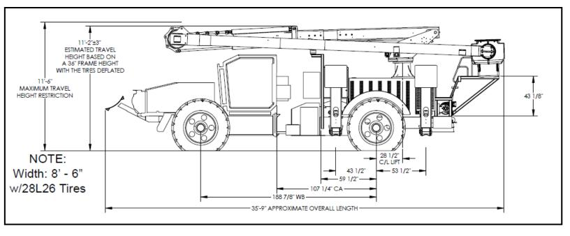
**Description:** The ATC7 is an all terrain, rubber-tired vehicle capable of supporting various aftermarket attachments. The machine is specifically designed for the vegetation management industry. Provides easy access to remote areas of utility, highway, and railroad right-of-ways.
