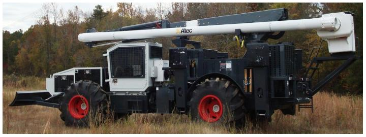
Currently Altec's bucket is a self contained unit with: Kubota pony engine Air compressor Auxiliary hydraulic tank. The 11'2" minimum height is accomplished by letting air out of the tires.
