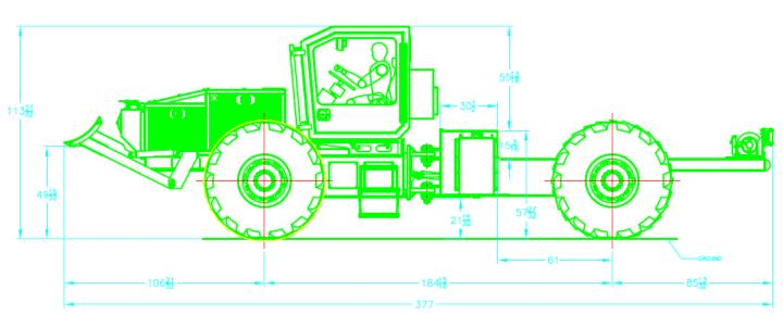
Weight: 18,000 lbs. carrier only. Width dimension shows 28L26 tires in work position. Tires can be moved in to 8'6" for trucking
