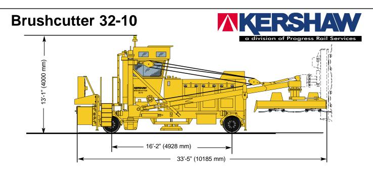
**Description:** The Kershaw 32 clears brush and overhanging branches from railroad right-of-way. It is capable of cutting up to 30 ft. (9144 mm) from the track center, and leaves behind a biodegradable mulch.
