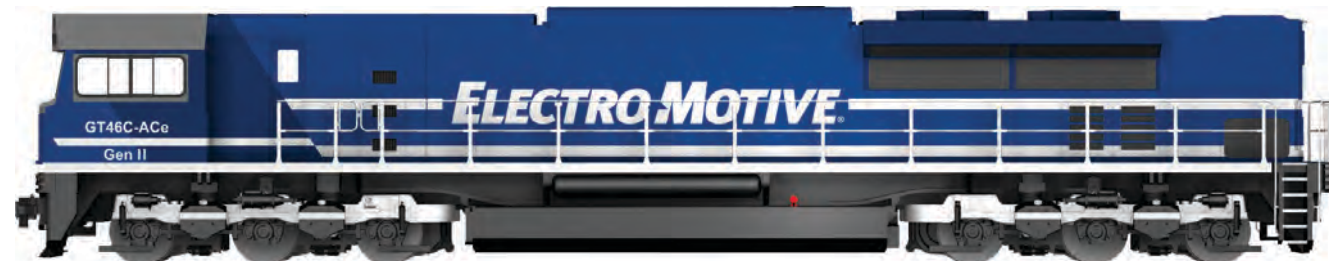
GT46C-ACe Gen II 180 Tonne with 12,000 L Fuel Tank, SD70ACe (HTSC) Bogies, and #2 End Platform
