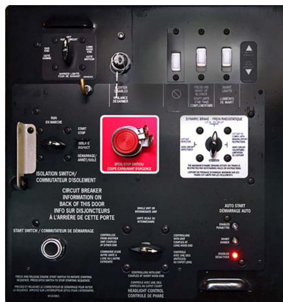
Photo depicts the AESS status portion of the engine control panel.
