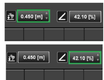
While adjusting depth and slope, target values are displayed.
