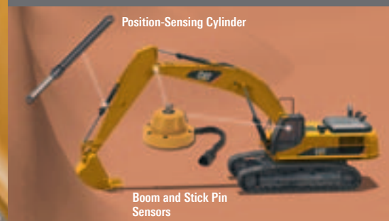
INTEGRATED SENSORS Embedded sensors, protected from damage
