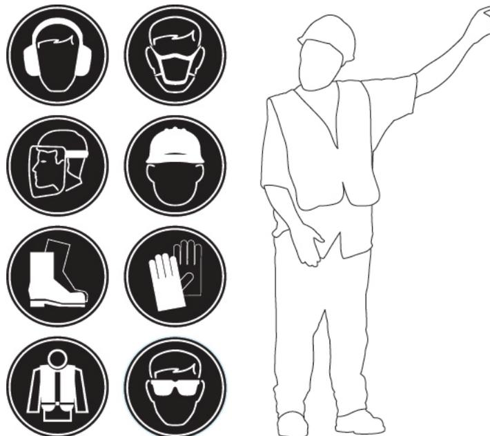
Figure 2.1 – Typical PPE to be worn by an Operator
