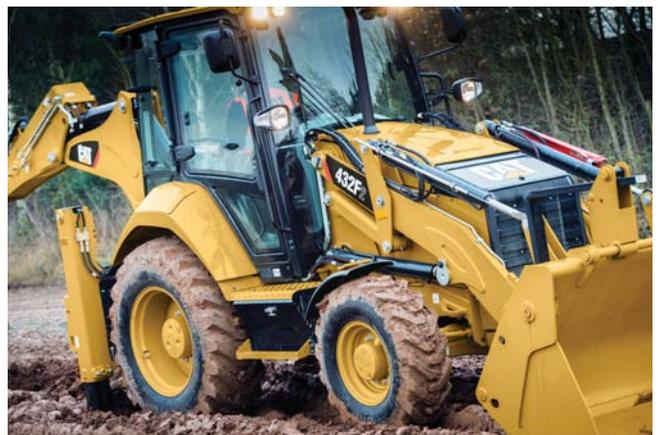
The 432F2 is fitted with pilot controls providing low effort operation, with the ability to switch between ISO (Excavator) or SAE (Backhoe) control patterns with the press of a button. Providing easy and safe operation for operators of any experience or ability.
