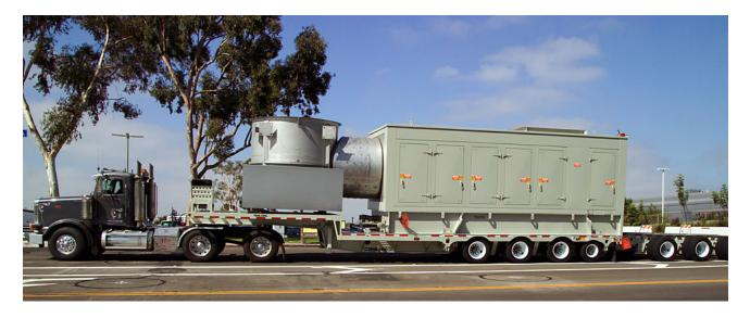
The Titan<sup>™</sup> 130 Mobile Power Unit is the prime choice if you're looking to produce reliable, low-cost, onsite continuous duty or peaking power. Designed as a complete power plant, the Titan 130 Mobile Generator System includes these key features:
