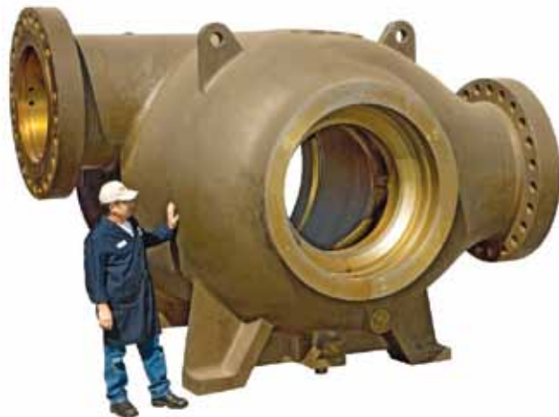
C85 Gas Compressor
