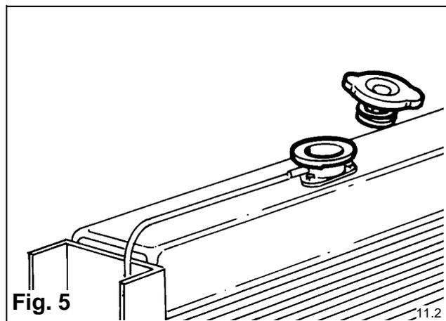
The use of plain drinking water is not recommended owing to chemical reactions which can result in corrosion and furring-up of the cooling system. A solution of either water and universal anti-freeze or water and corrosion preventative must be used. Refer to **page 17**.
