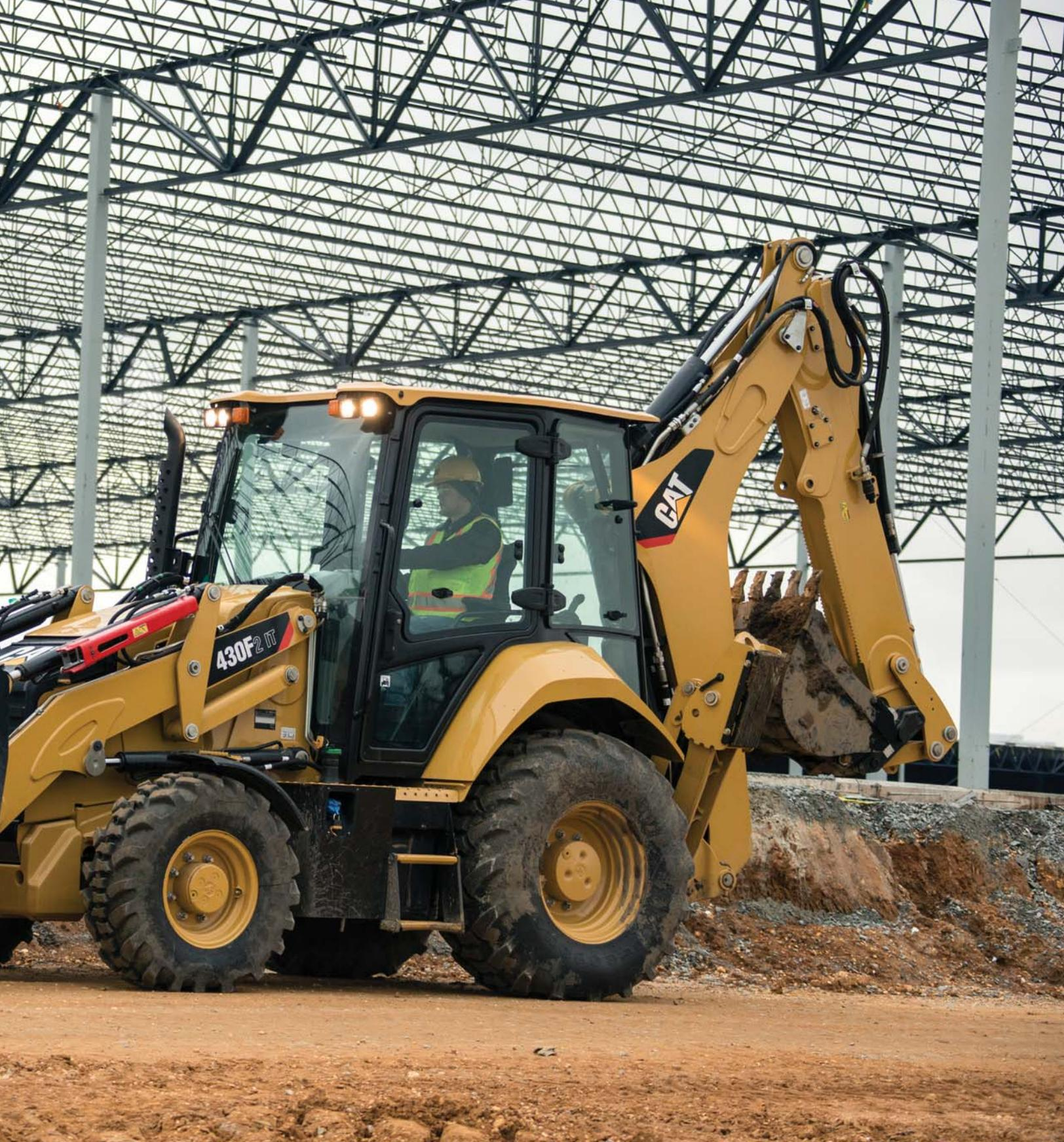
**Experience the Backhoe Loader designed around customer feedback. The Cat 430F2 Backhoe Loader puts all the machine controls at the operator's fingertips. Operate all auxiliary controls with thumb rollers. Move from job site to job site quickly and smoothly with the additional 6th gear on the autoshift transmission and optional lock-up torque converter.**
