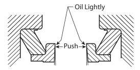
After installing the seal halves into the unit, wipe both metal sealing faces clean with a lint-free wipe. Apply a thin film of oil to the sealing faces with a lint free applicator. Oil must not contact surfaces other than the sealing faces.
