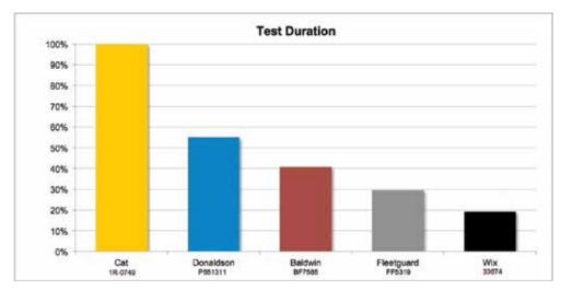
The Cat 1R-0749 Advanced High Efficiency Fuel Filter was pitted against (4) equivalent competitive filter brands to compare injector life. Two filters for each brand were tested and the results averaged together to show the performance for each brand. The injectors with Cat filtration lasted 45% longer than the nearest competitor.
