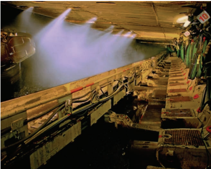
Cat longwall dust suppression system
