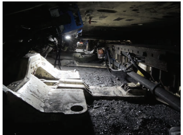
Cat roof supports specifically designed for low-seam operation
