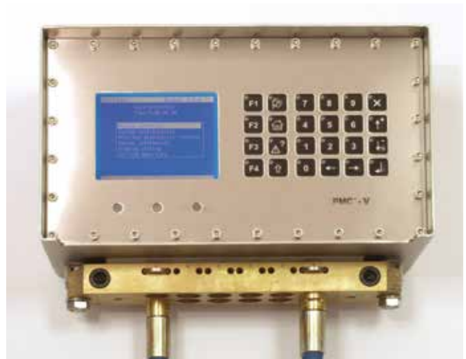
PMC-V – mainly for visualization of data and parameter settings
