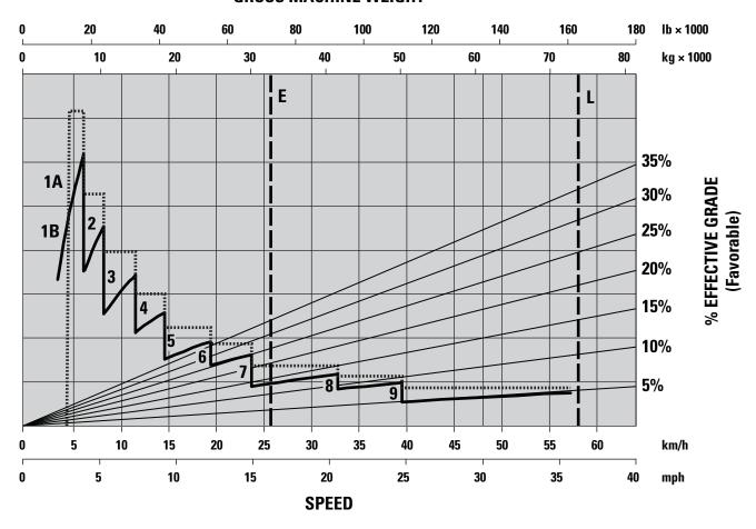
1A – 1st Gear (Converter Drive)
