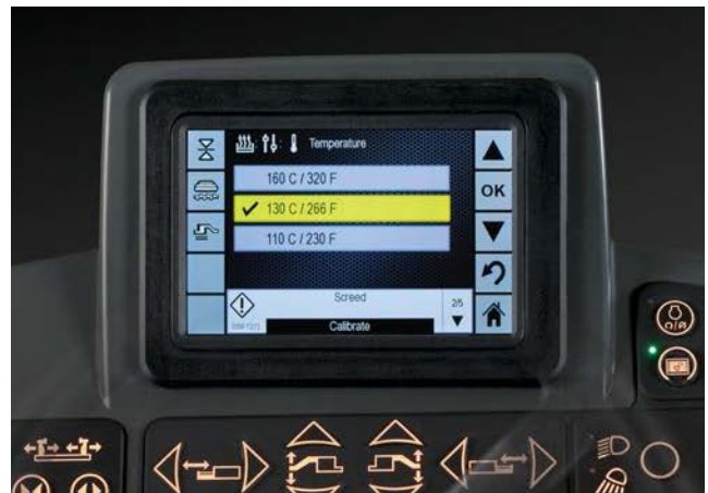
Three preset heating options provide a wide range of temperatures for various mix designs.
