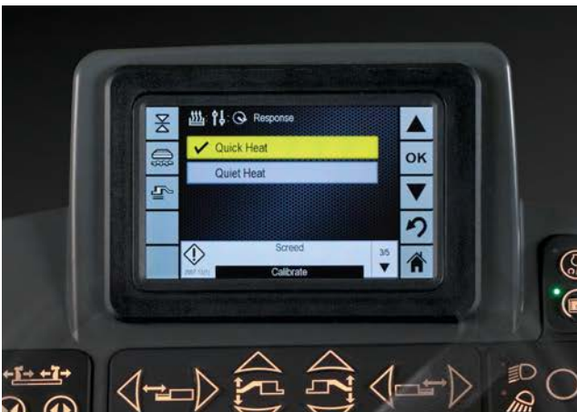
Quiet or quick heating made easy through the LCD display. Quick heating offers time-savings when utilizing wide-width packages.
