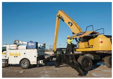
Primary service points are easily accessible through convenient panels and platforms on the sides and top of the machine.
