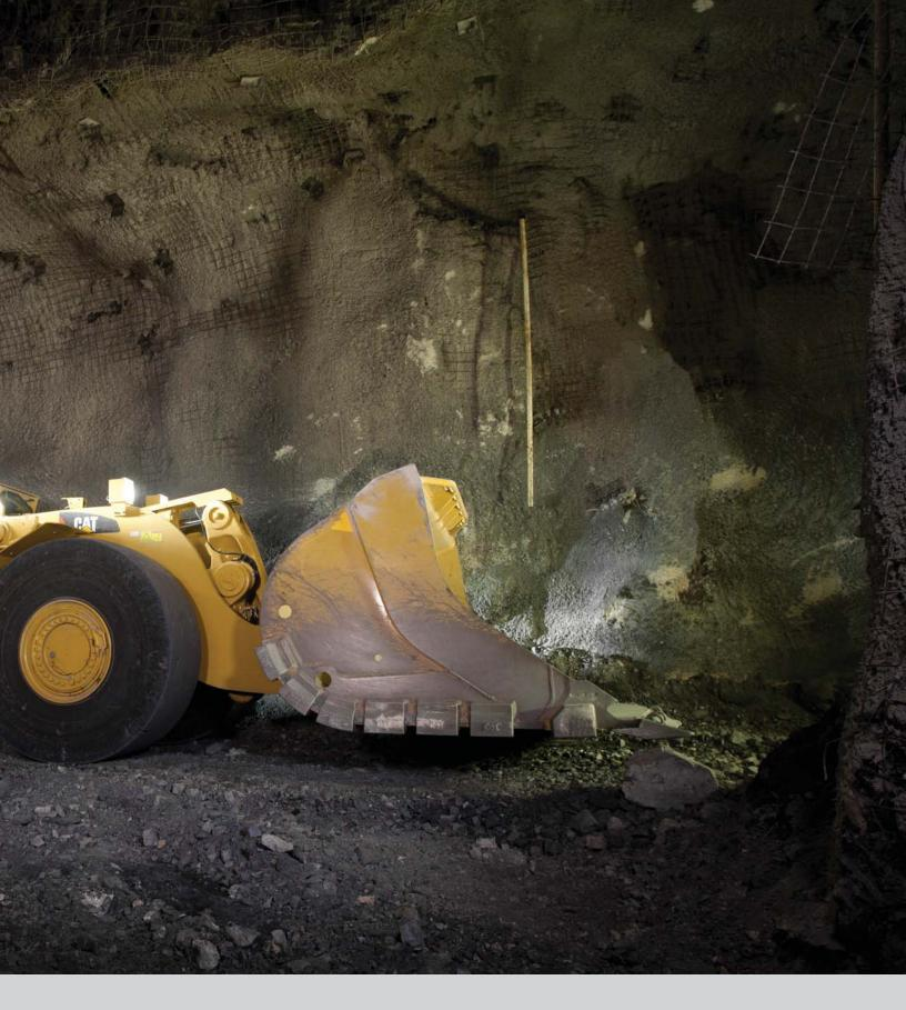
Command for underground enables remote operation of load-haul dump machines. Developed out of the need to reduce human exposure to injury, the system removes the operator from hazardous environments and allows them to work in a safer, more comfortable, ergonomic operator station. Command for underground increases productivity and safety, making a measurable impact on your mine's bottom line.
