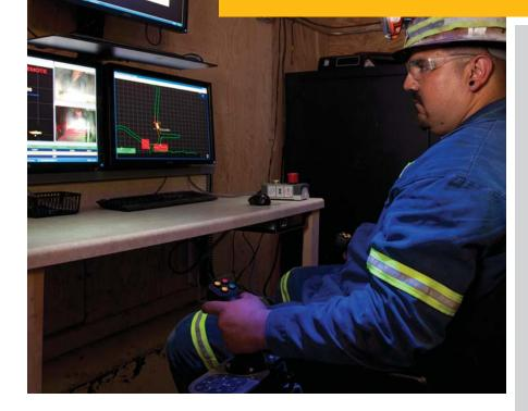
The operator station allows machines to be operated from an ergonomically designed seat in a safe control room environment. It can be mobile or in a fixed location either underground or on the surface.
