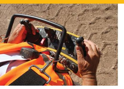
The operator console allows for line of sight control of up to 400 meters (437.4 yd) with the option of a 900 MHz version or a 2.4 GHz version. The console and on-board transceiver utilize spread spectrum technology to virtually eliminate interference from other wireless devices utilizing the 900 MHz or 2.4 GHz frequency bands. Proprietary algorithms secure the communications between the on-board wireless receiver and the console, preventing communications from unauthorized devices.
