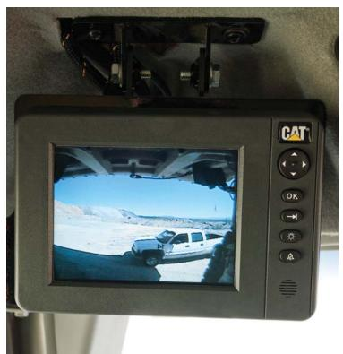
At the most basic level, Detect enhances your operators' awareness of the immediate environment around their equipment through a simple camera and touch screen display system, called Vision. This system is scalable, allowing radars to be added that provide alerts to operators when objects have entered critical areas near the machine. The system allows a quick visual check of these areas whenever needed by the operator.
