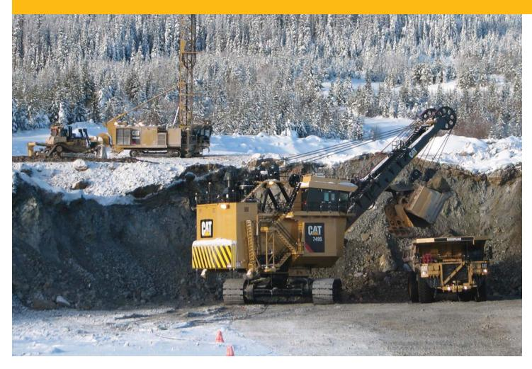
Proximity Awareness is a GNSS based system that tracks machines and light vehicles, allowing operators to view other machine locations and provide proximity based alarming.
