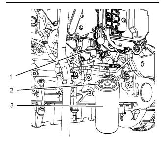
4. Apply clean engine oil to the O ring seal (2) on the new oil filter.
