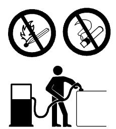
Use caution when you are refueling an engine. Do not smoke while you are refueling an engine. Do not refuel an engine near open flames or sparks. Always stop the engine before refueling.
