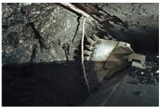
The lower the coal seam the more difficult it is to mine, so loading the coal onto the Armored Face Conveyor (AFC) becomes ever more important in lower seams. The plow body of the Cat GH800B has an optimized design that allows it to load more coal onto the face conveyor and reduces the amount of cutting power wasted in the process. The new shape at both ends of the plow body and the lower height of the plow guide significantly improve the coal loading process in low seam heights.
