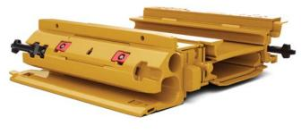
The plow guide of the GH800B — which connects the plow body to the conveyor — is made out of a one-piece casting. This provides extra strength and durability while being much lower in height than the old welded plow guide. The casted plow guide can withstand the high reaction forces on the line pans from the powerful AFC drives.
