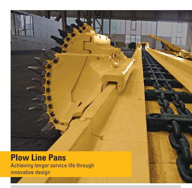
One feature maintained by the new GH800B plow system is the Cat AFCPF3 or AFCPF4 conveyor, which uses plow line pans with a replaceable top trough for easy replacement of worn-out parts. They also feature external dogbone connectors between the line pans — each with a breaking strength of up to 3600 kN (404 tf), as well as a very strong and flexible relay bar between the conveyor and the roof supports.
