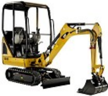
Mini hydraulic excavator Weight = 3241 lbs.
