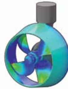
Hydrodynamic optimization by CFD simulations
