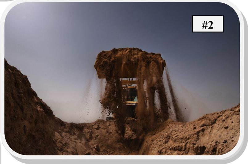
3. The bulldozer is providing additional power from behind helping the scraper move forward.
