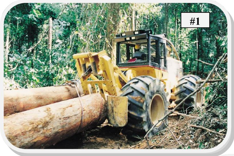
1. The 545C Wheel Skidder drags logs to the staging area for processing.
