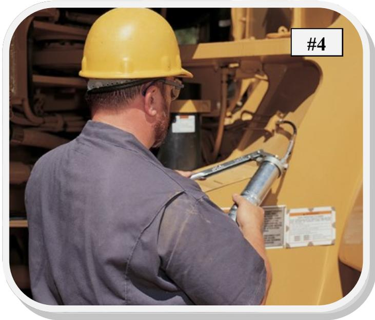
4. The service technician is applying a lubricant with a grease gun.
