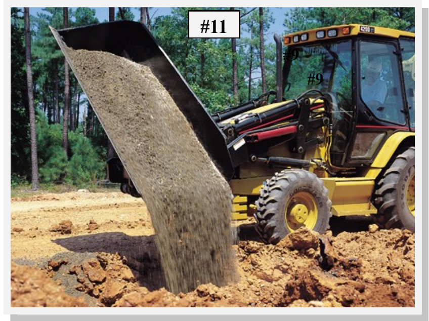
11. This backhoe has a bucket that will dump to the side.
