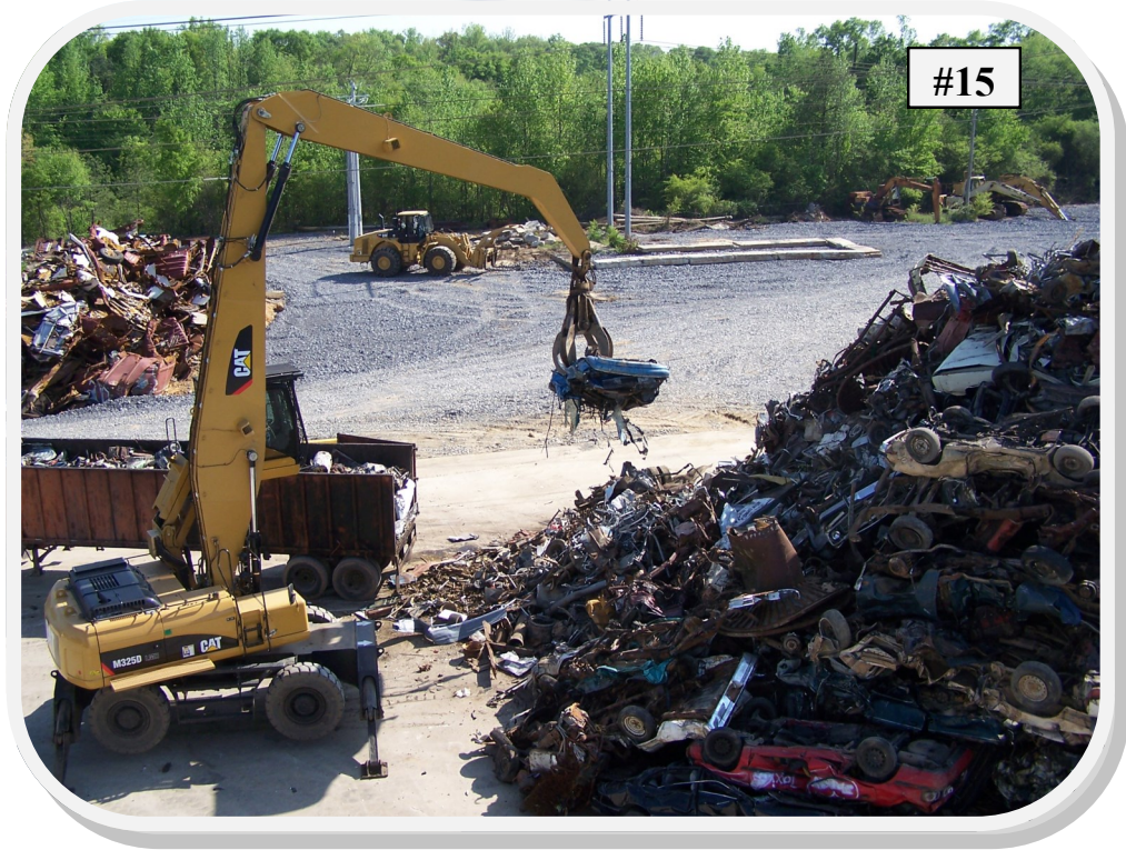
The M325D Material Handler picks up scrap to load the semi trailer.
