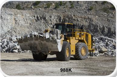
The 988K Wheel Loader has a 12.5-ton rated payload capacity. The 990H has a 16.5-ton rated payload capacity.
