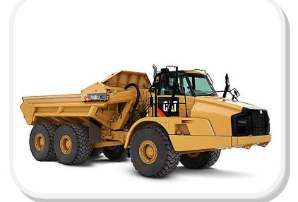
A ton of bricks weighs 2,000 pounds. The 740B Articulated Truck has a 42-ton payload capacity.
