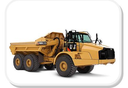
A ton of bricks weighs 2,000 pounds. The 740B Articulated Truck has a 42-ton payload capacity.
