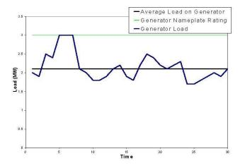
Figure 1: Example Load Profile – 3 MW Standby Rating
