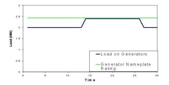
Figure 6: Example Load Profile – 2.5 MW Continuous Rating
