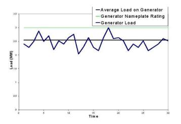
Figure 2: Example Load Profile: 3MW Mission Critical Standby Rating
