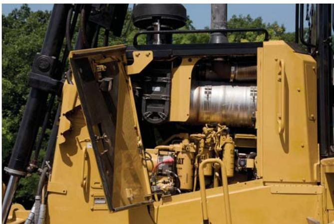
Emissions reduction technology on the D8T is designed to be transparent, with no action required from the operator. Regeneration runs automatically in the background while you work.
