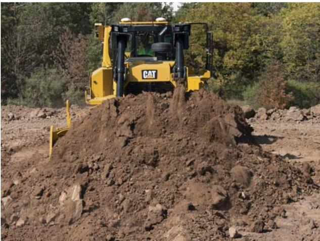
The integrated design moves the antennas to the top of the cab, eliminating masts and cables traditionally on the blade. 3D mapping of blade and tracks reduces the need for grade checkers and staking, enhances safety and reduces labor costs.
