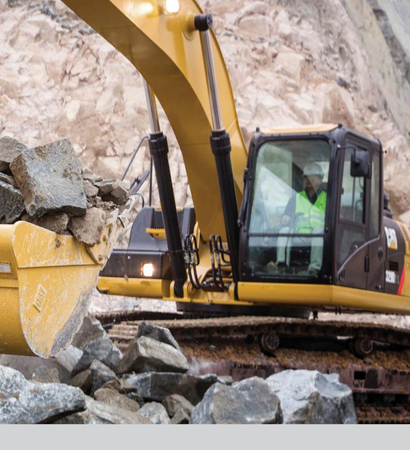
The 329D2/D2 L comes with a number of new developments and features to help you make the best use of your machine including, isochronous engine speed control, a new fuel filtration system, a built-in economy mode to reduce fuel consumption by up to 11 percent. A variable speed fan with viscous clutch makes this machine productive, efficient, and safe.
