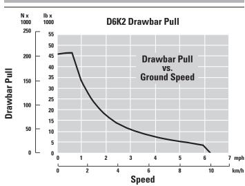
• The direct injection electronic fuel system provides a controlled fuel delivery increase as the engine lugs back from rated speed. This results in increased horsepower below rated power. A combination of increased torque rise and maximum horsepower improves response, provides greater drawbar pull and faster dozing cycles.
