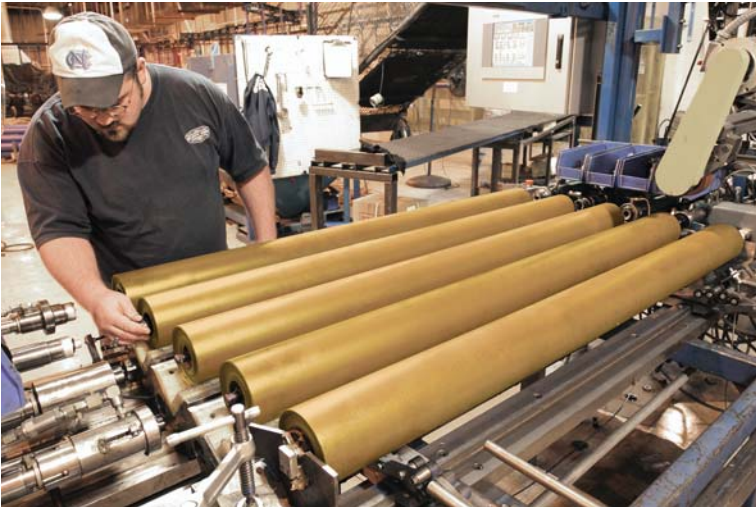
Cat steel® rolls go through an automated five-stage assembly and testing process.
