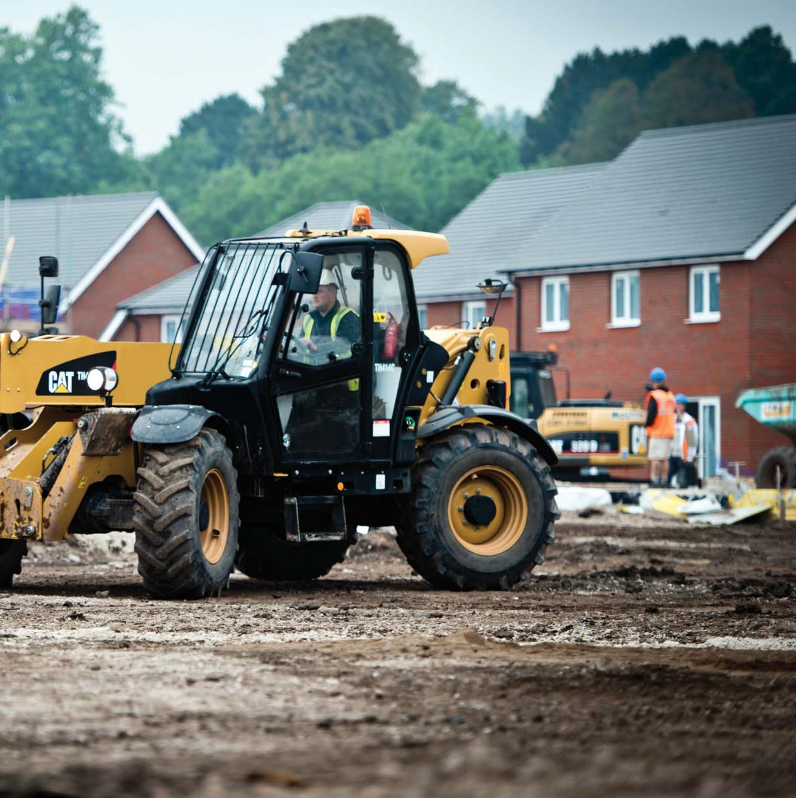
**The C Series Telehandlers have a new engine to meet EU Stage IIIB equivalent emission standards and a new powershift transmission that ensures the operator can easily select the right ratio for the job in hand.**
