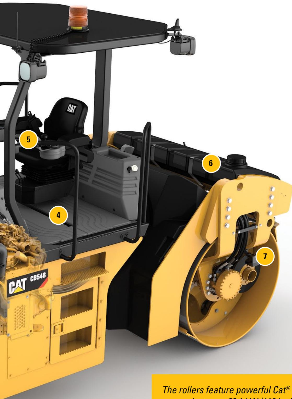
*The rollers feature powerful Cat® diesel engines, with ranges between 82.1 kW (110 hp imperial, 111.6 metric hp) and 96.5 kW (129 hp imperial, 131.2 metric hp).*
