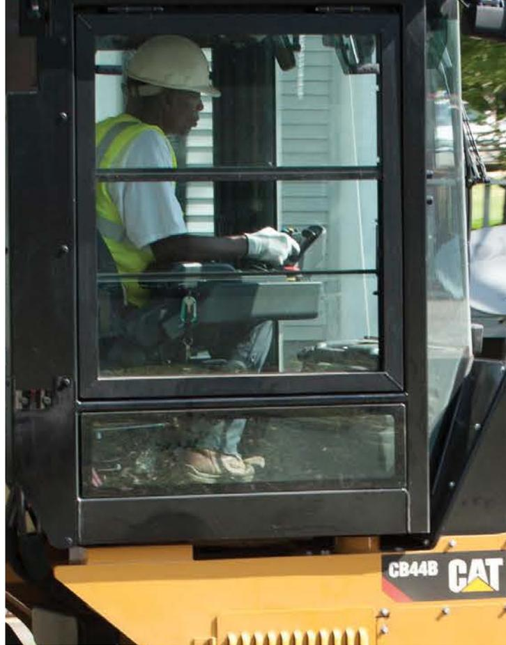
*Cat control consoles are integrated with pivoting seats, keeping controls and the display right at your fingertips.*
