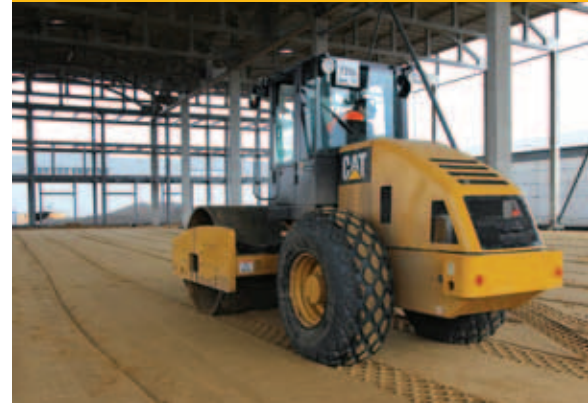
▲ The CS533E Vibratory Soil Compactor at work in a future warehouse.
