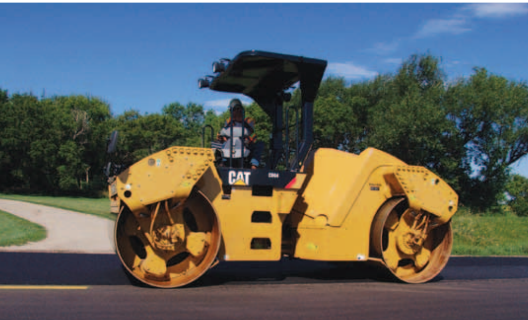
^ An operator selects the frequency with the flip of a switch.
