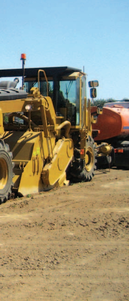
▲ The RM500 rotary mixer and its feed truck are followed by the Cat Motor Grader.
