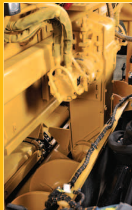
^ Variable speed augers deliver an even head of material.
