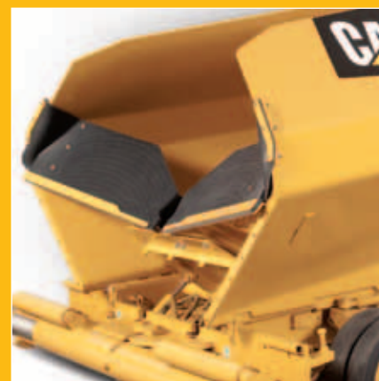
^ The foldable front apron and optional hydraulic lift simplify cleanout.
