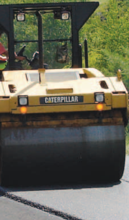
^ 2 m (79") Cat compactor working in the hottest temperature zone staying ahead of the tender zone.
