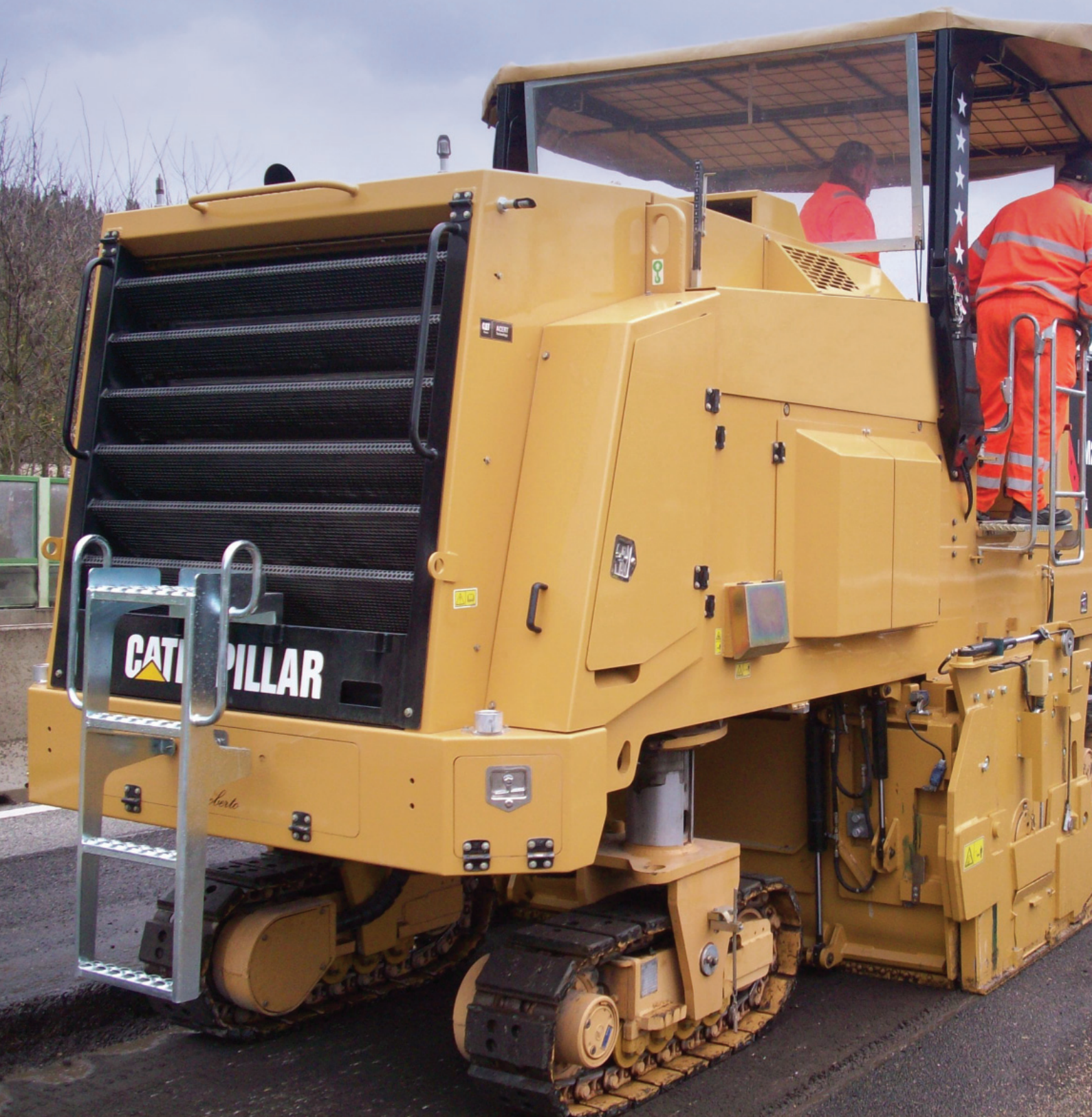
^ The 2.2 m drum enabled the crew to mill Motorway E78 in four passes instead of five.
